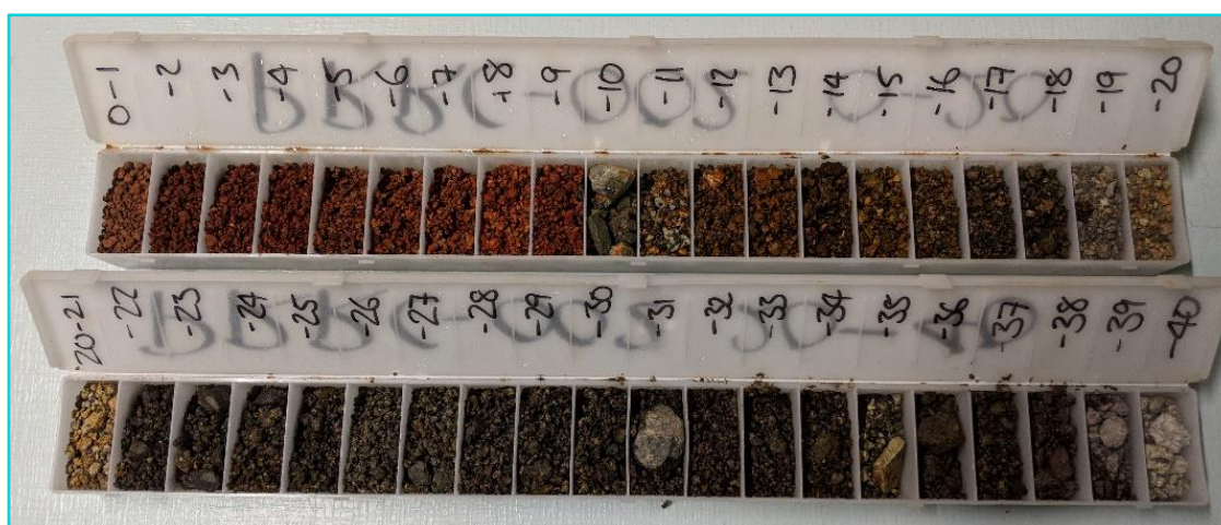
Figure 1 - RC chip tray from hole PRRC002 with 18m @ 1.85g/t 3E PGM from 20m
