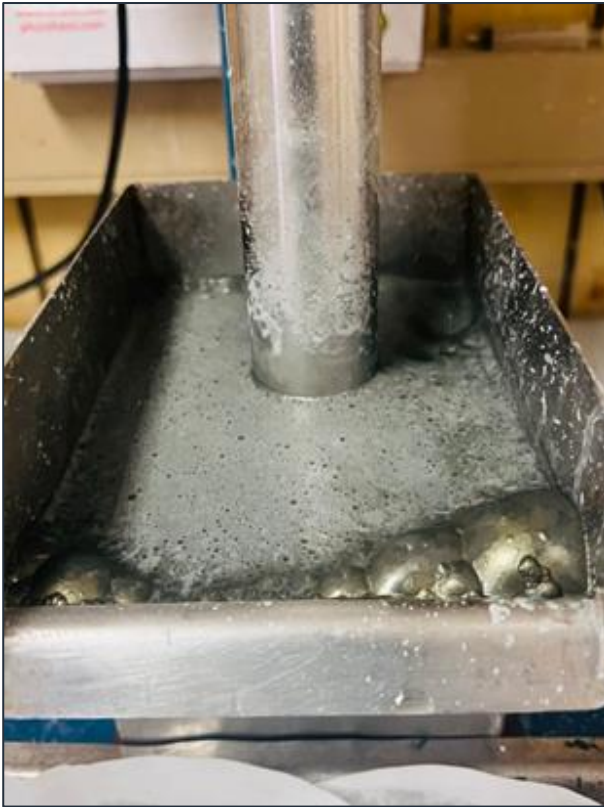
Figure 2 – Typical flotation of Parks Reef ore (left) and rougher concentrate from laboratory flotation test (right)
