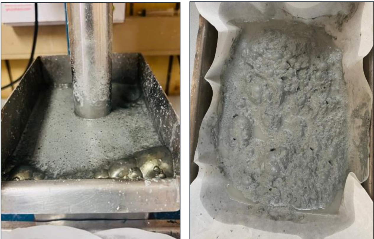
Figure 2: Typical flotation of Parks Reef ore (left) and rougher concentrate from laboratory flotation test (right)
