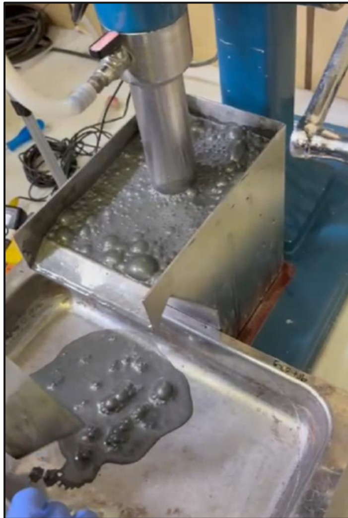
Figure 1: Flotation test producing high-value rougher concentrate
