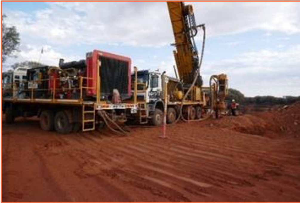
Figure 4 – RC Drill Rig in Operation on the Stage 10 Programme.
