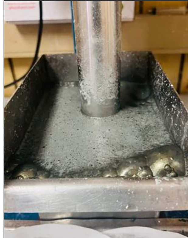
Typical Flotation test producing Rougher concentrate
