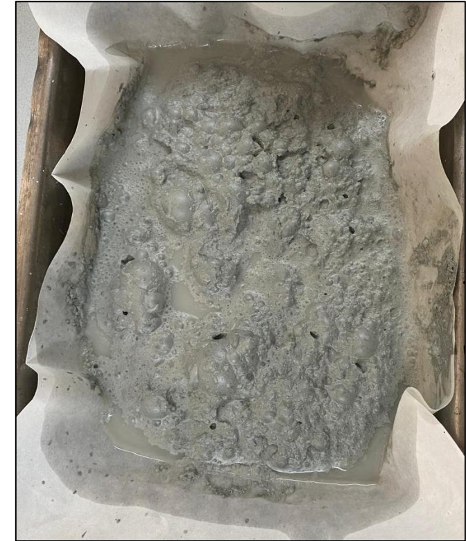
Rougher concentrate from laboratory flotation test
